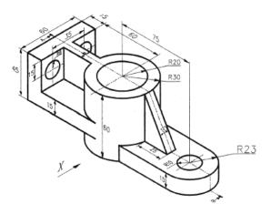
b) Draw the isometric view of the object, the orthographic views of which are shown in the figure below.
